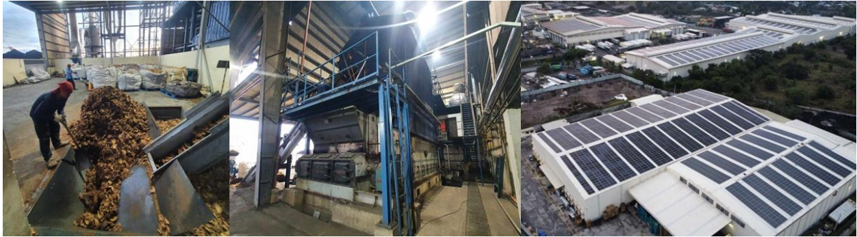
(Pictured, Left to Right) 1. A worker at CNPF's Coconut plant scoops up coconut by-products. 2. Boiler 5, its newly commissioned biomass boiler. 3. Solar PV panels on the rooftop of CNPF's manufacturing hub in General Santos City
